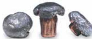
Lead core is bonded to pure copper jacket
