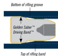
The bullet diameter directly ahead of the Driving Band™ is reduced from groove to bore diameter, so the bullet is precisely aligned before the Driving Band engages the rifling. The result: match-grade accuracy and reduced barrel friction that conserves velocity.
