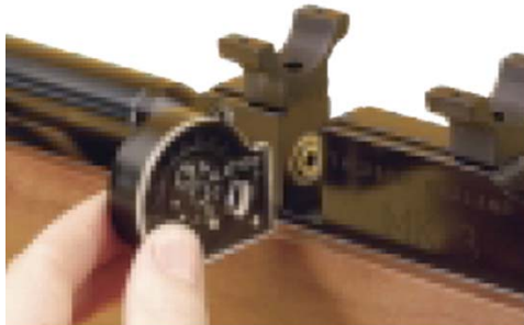
The 12 and 17 shot magazines fit in from the left hand side of the rifle. Make sure the magazine clears the scope turrets.
