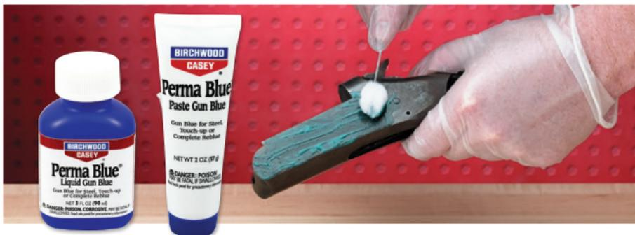
2 Allow the blueing to stand on the metal for **30-60 seconds**. **No longer.** Then neutralize the chemical reaction by rinsing immediately and thoroughly with **cold** water and wipe dry (💡Read Carmichel's Tip below).
