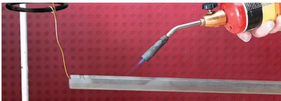
**2** Heat evenly by moving the heat source back and forth along the item being browned. Note that heavier areas (like the barrel breech) will take longer to heat and will retain their temperature longer. Also, small parts are more likely to get overheated. So heat thoroughly to 275°F. To test the temperature 🔦Read Carmichel's Tip below. It is not necessary to heat the entire barrel at the same time. The barrel may be heated and finished in sections.
