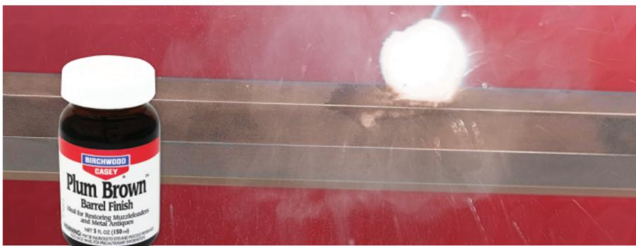
3 When the ideal temperature of 275°F has been obtained, apply Plum Brown Barrel Finish with a saturated swab in long even strokes. The rich plum brown color will appear immediately. (💡Read Carmichel's Tip below).
