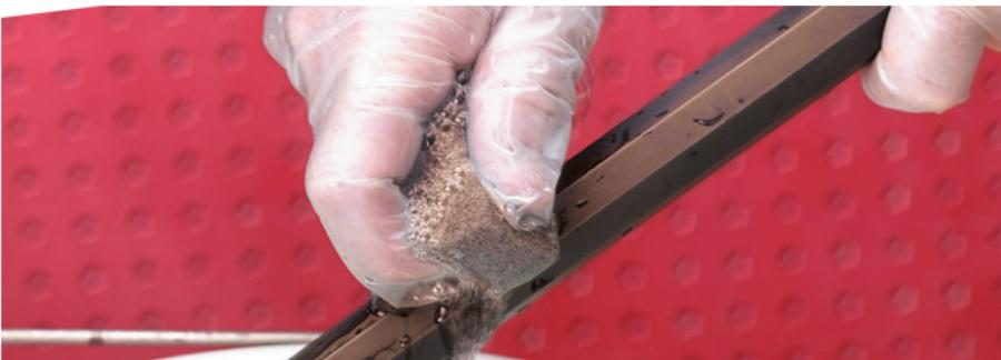
**6** When browning is complete, rub all surfaces down with Barricade Rust Protection. This is very important after rinsing and will penetrate the surface and give you a deep, rich, mahogany-brown permanent coating. Allow to cure for 24 hours.
